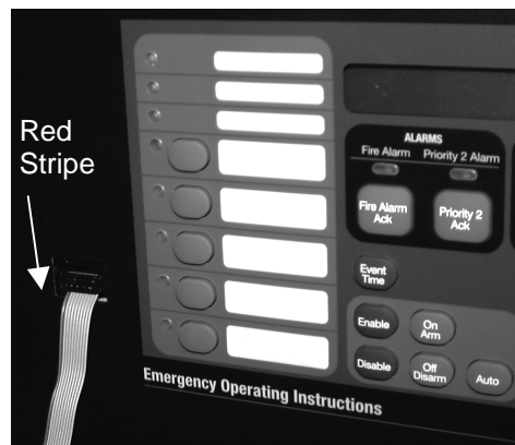
Figure 14-3. Connecting the 733-794 Cable to the Panel
