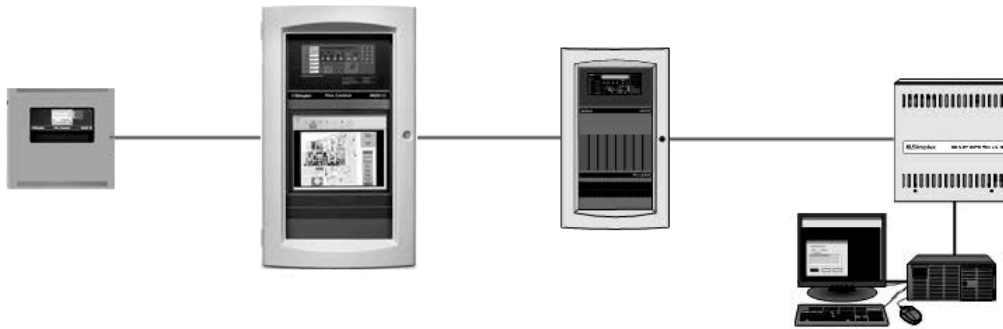
Figure 6: Single run linear network topology. No T-tapping.
