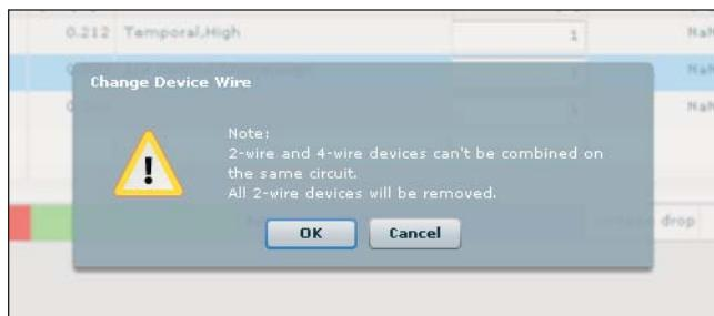
Also in a circuit user can not combine 2-wire devices and 4-wire devices, hence when user tries to change the wire type either in step 3 to add devices or in the grid section using Wire Type combo box, user will be given a message as seen left.
