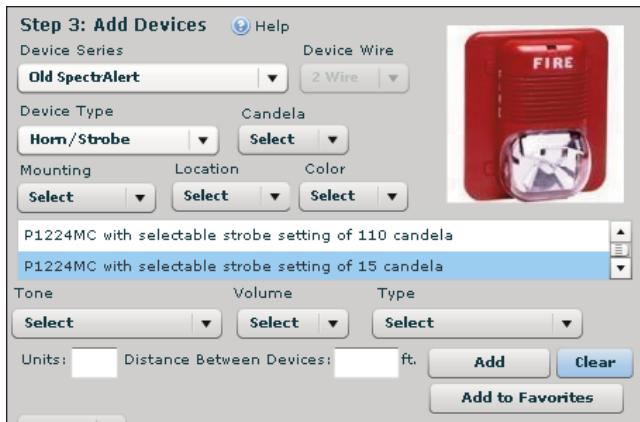
Above selection of P1224MC with selectable strobe setting of 110 candela uniquely selects a device and hence even if we do not select Mounting, location, or color, user will be allowed to add devices to the circuit.
